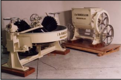
I. DeFrancisci & Son gramola (left), mixer (middle) and press (right) after refurbishment. The gramola and mixer were originally from Santoro Macaroni and later Bened Foods. The press was from V. LaRosa & Sons.
