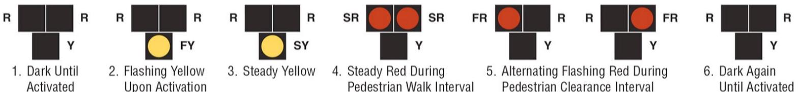
FY: Flashing Yellow • SY: Steady Yellow • SR: Steady Red • FR: Flashing Red
